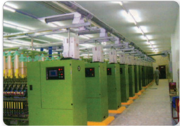
Cutes Inverter with Marzoli DTM 129 Ring Frame
