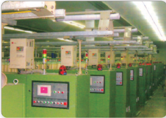
Cutes Inverter with Jing Wei FA 1520 Ring Frame
